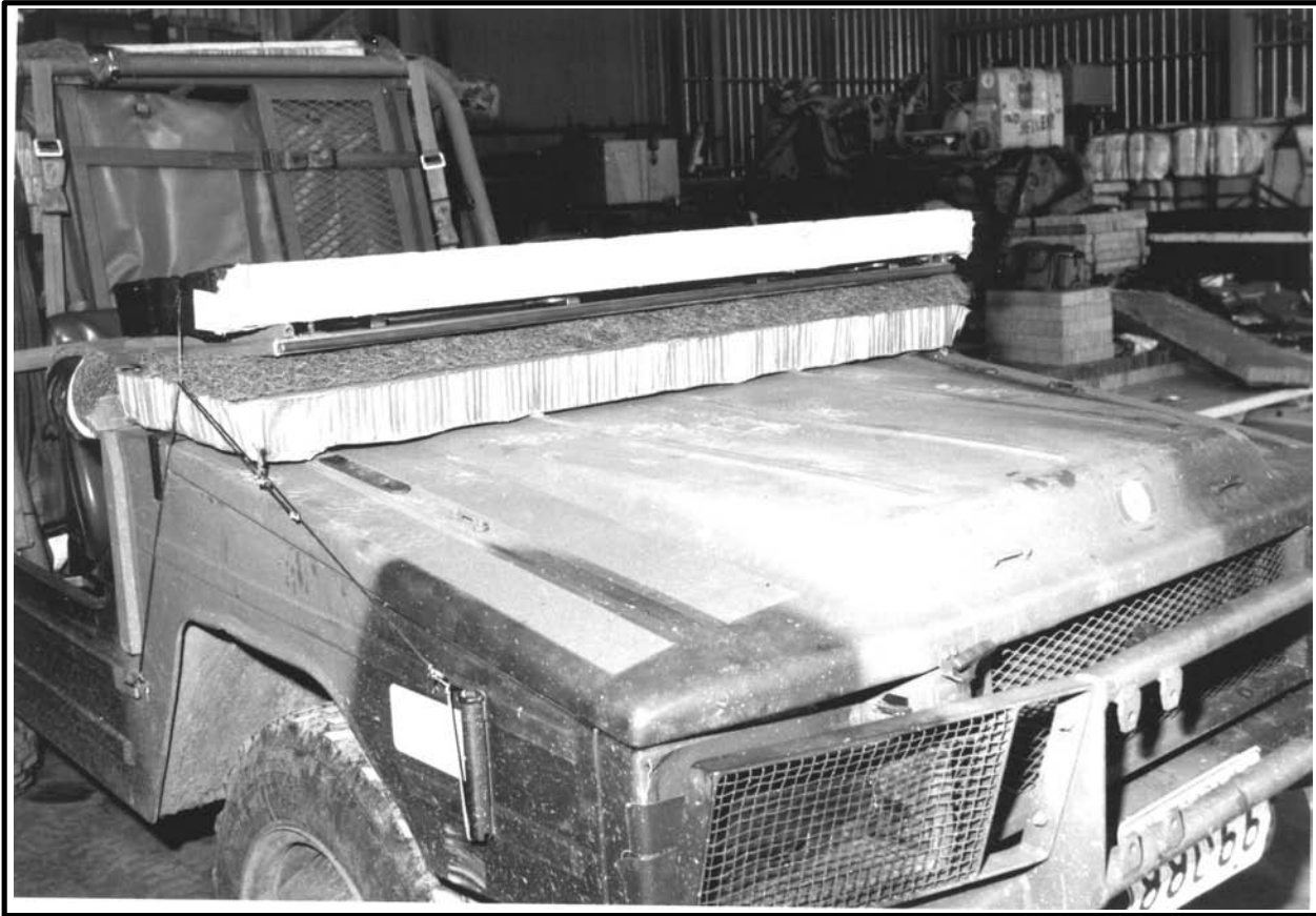
Figure 6-26 Windshield Protection Installed
