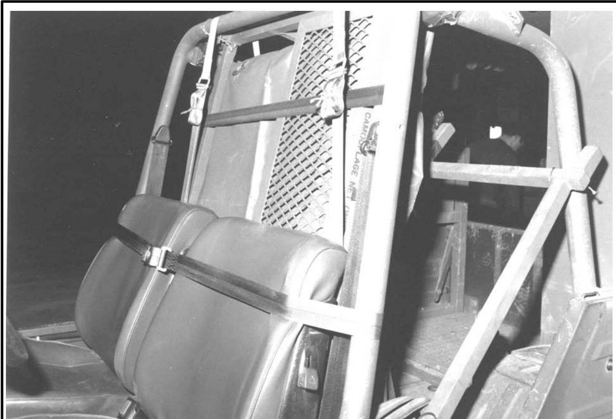
Figure 6-11 Roof Rack Positioned and Secured
