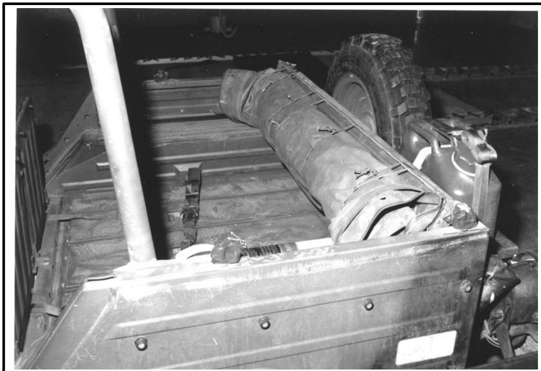
Figure 1-3 Rolled Tarp and Frame Secured
