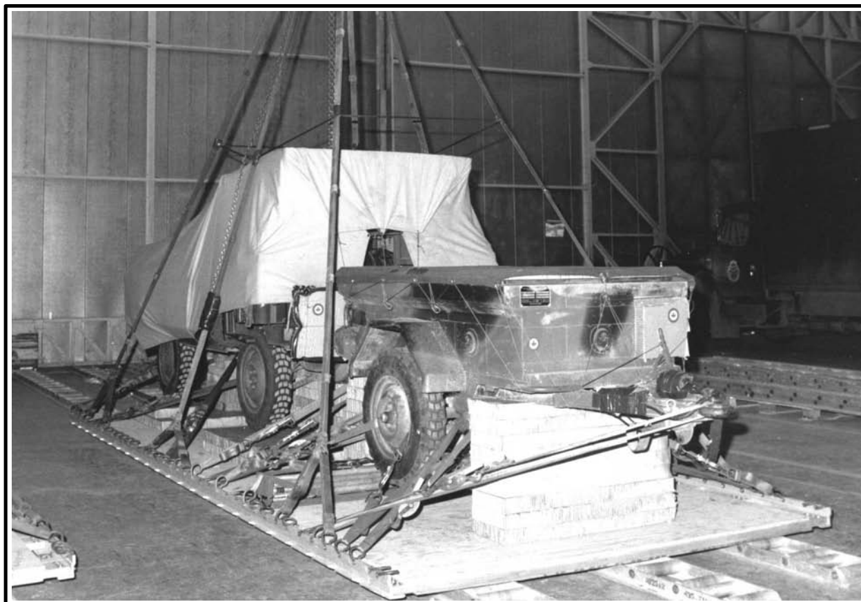
Figure 8-10 Suspension Slings Installed
