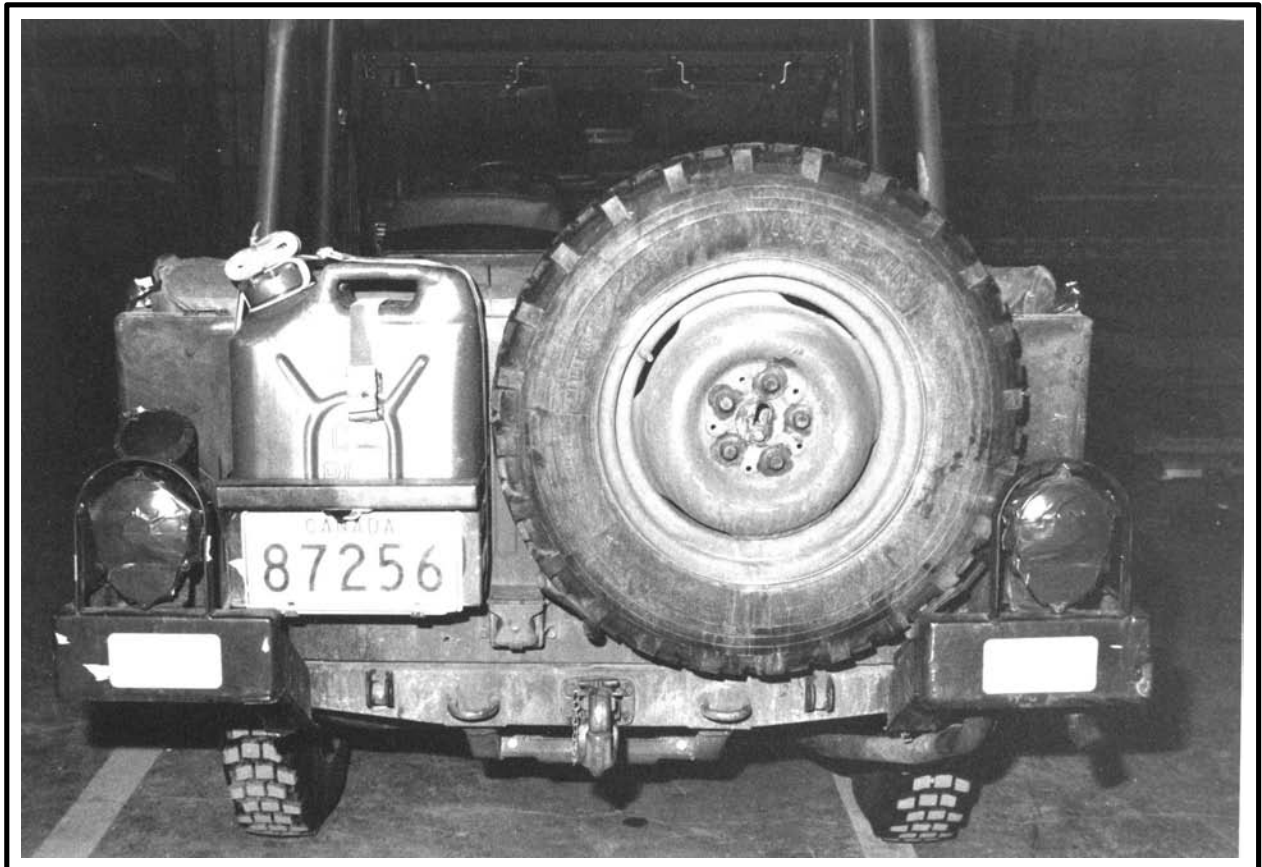
Figure 1-11 Gas Can and Spare Tire Secured
