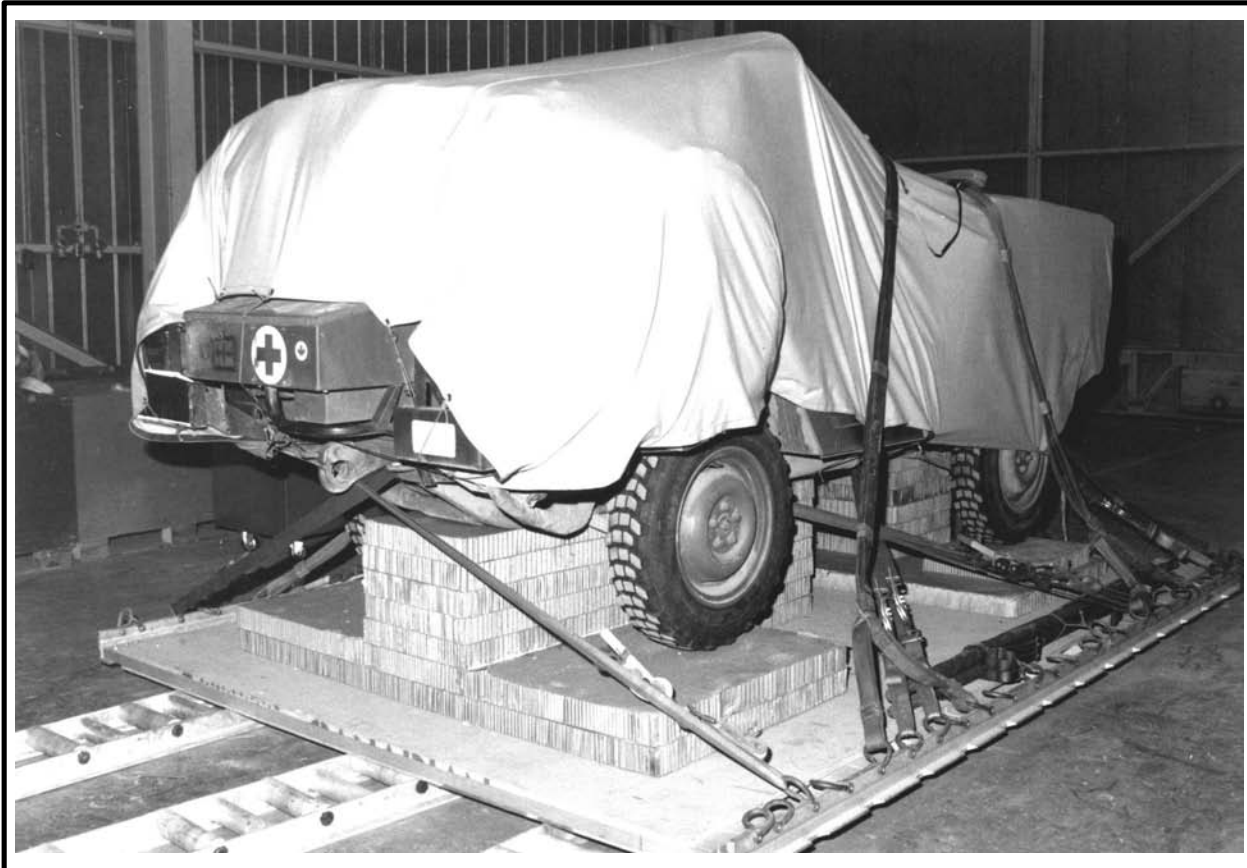
Figure 4-23 Installation of Canvas Cover
