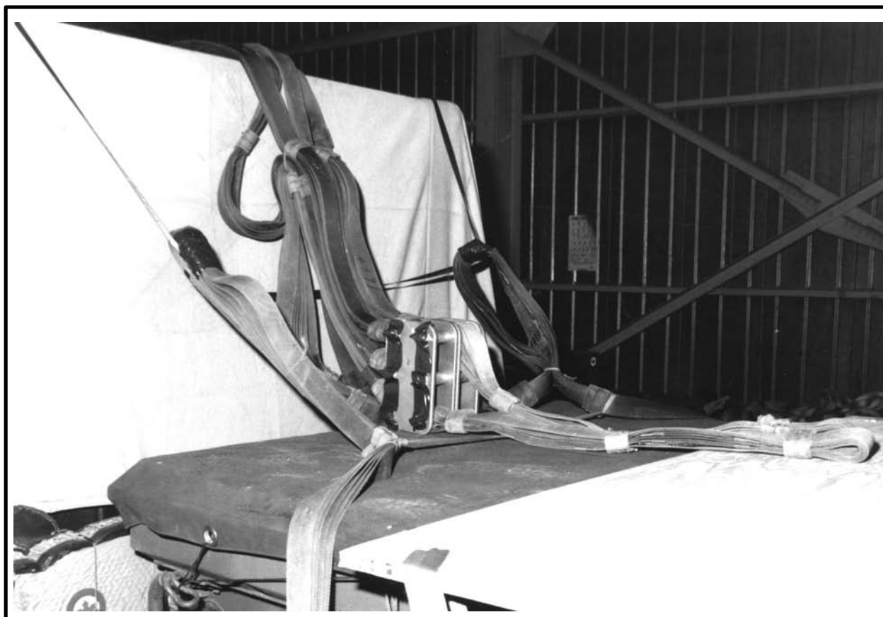
Figure 8-18 Suspension Slings Safe-tied
