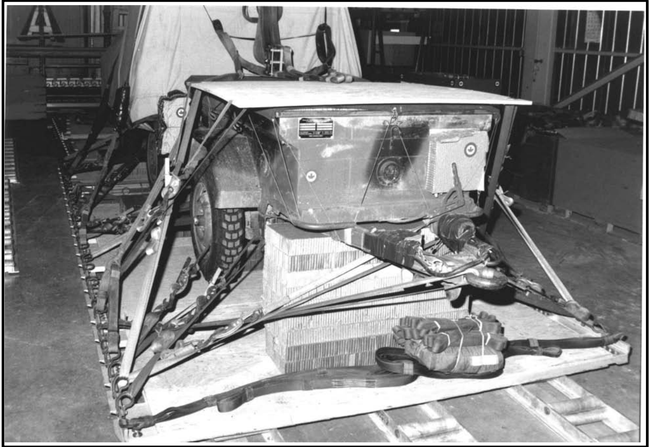
Figure 8-9 Parachute Tray Positioned and Secured
