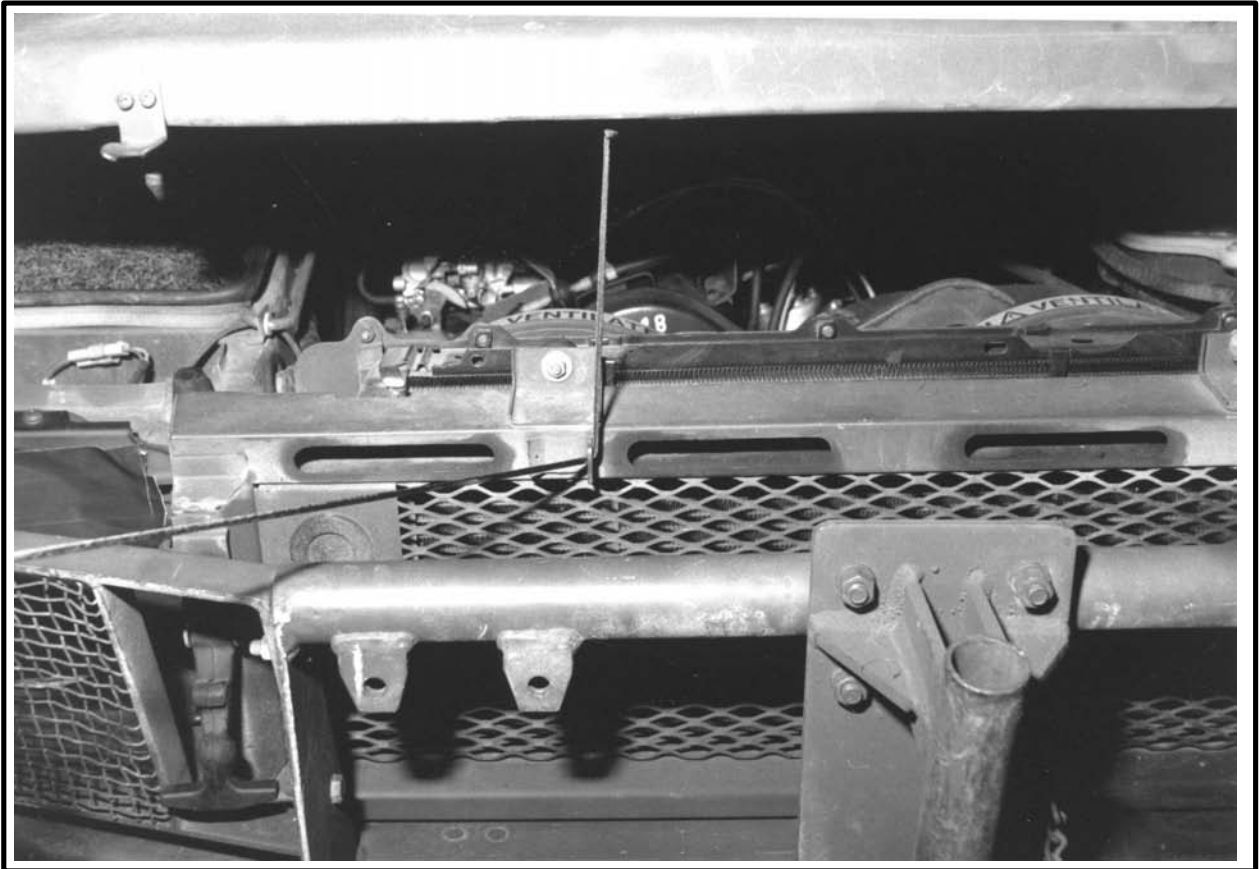
Figure 4-12 Type III Nylon Cord through the Locking Hole on Hood
