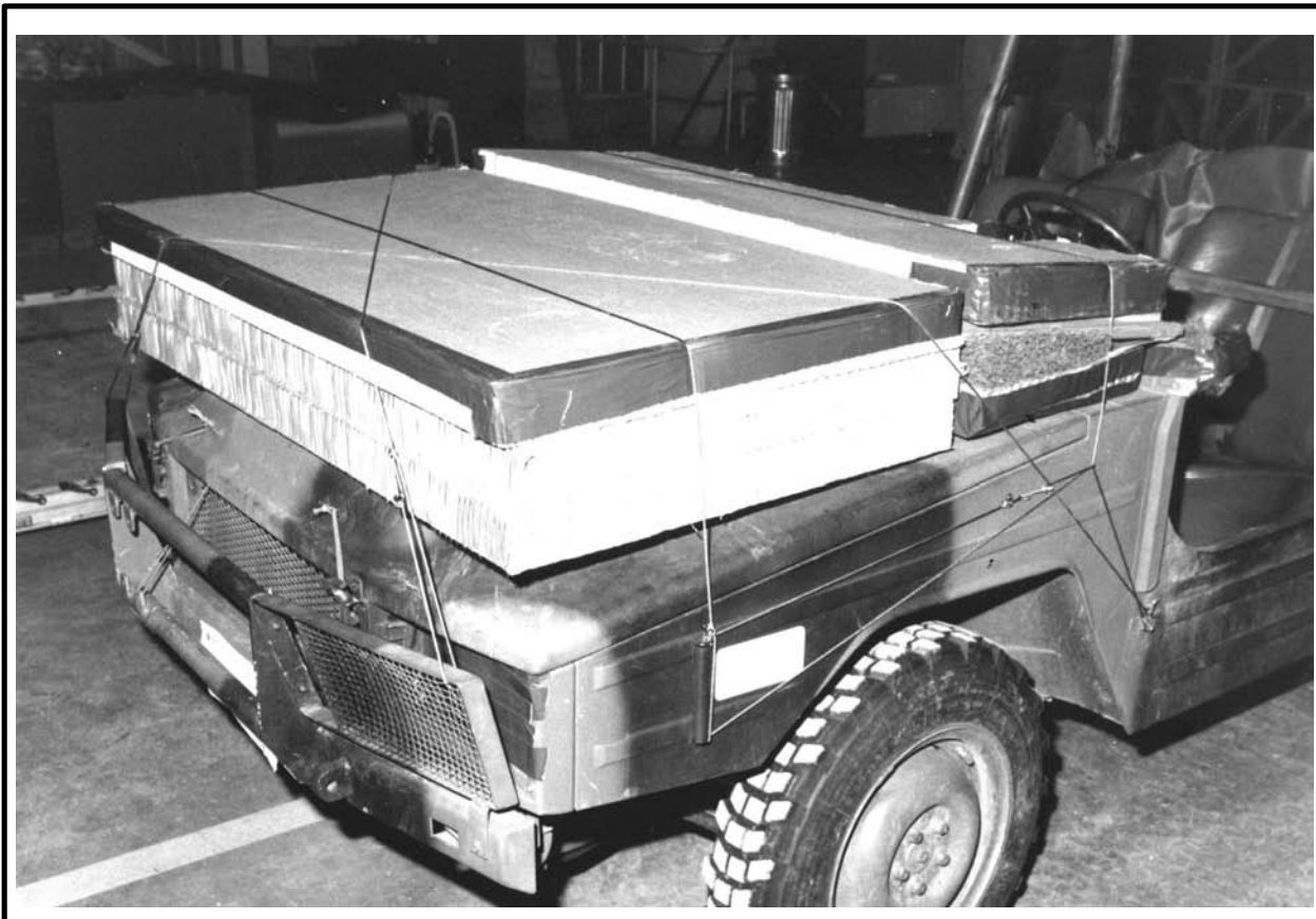
Figure 2-3 Parachute Tray Installed
