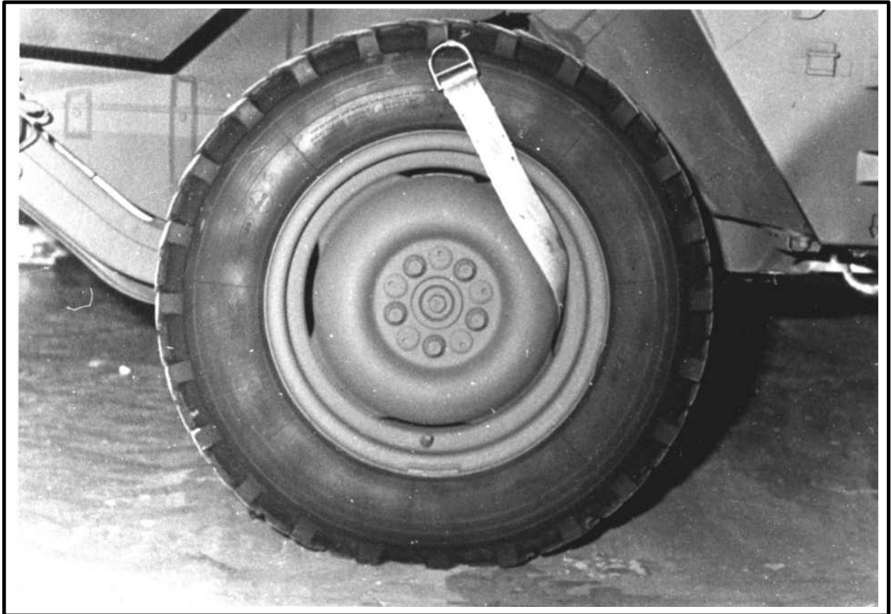
Figure 1-19 Strap Through Slot in Wheel Rim
