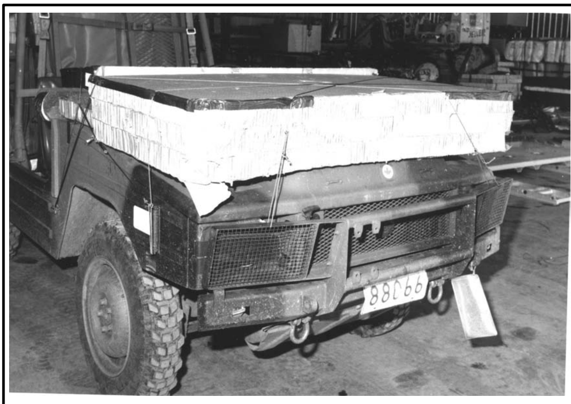
Figure 6-28 Parachute Tray Installed
