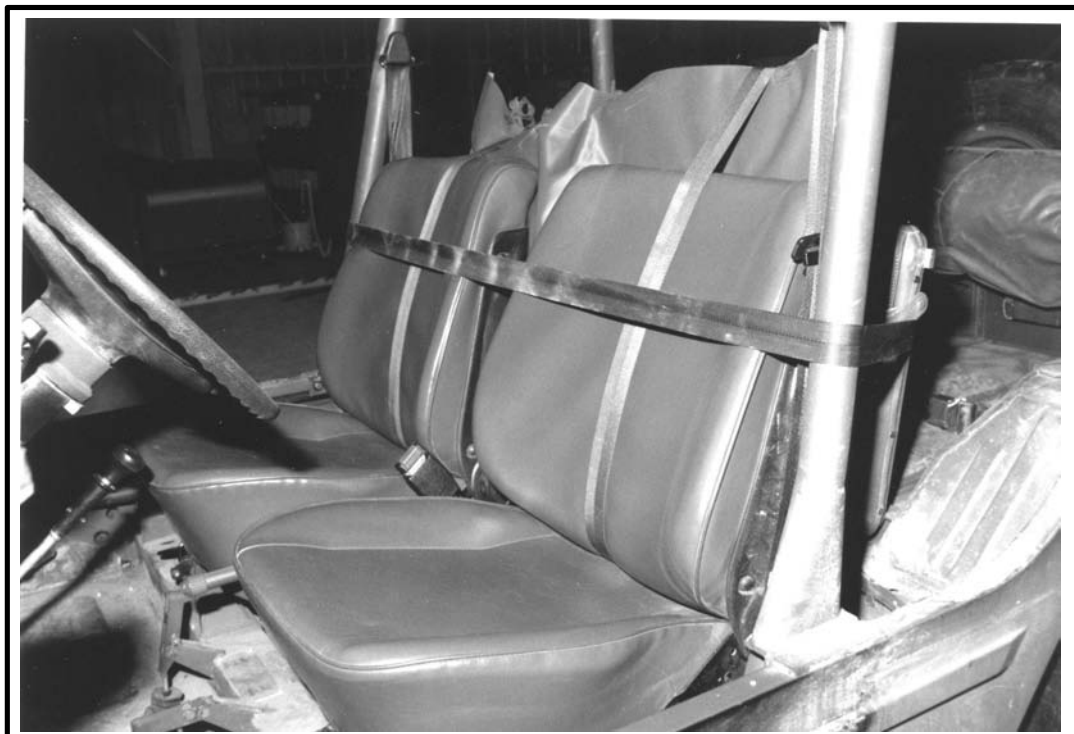
Figure 1-6 A7A Straps Installed (Front View)
