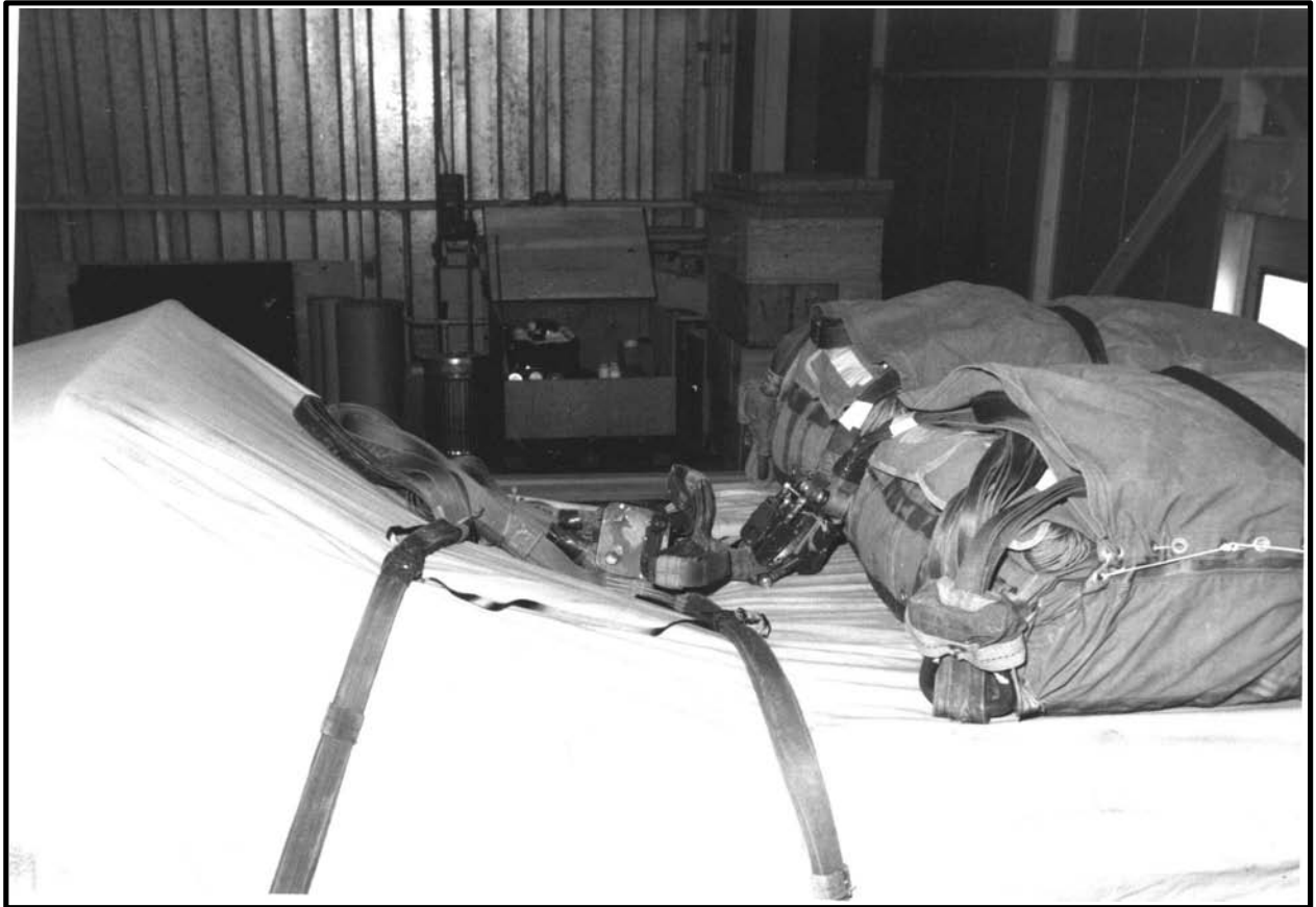
Figure 6-33 Suspension Slings Safe-tied
