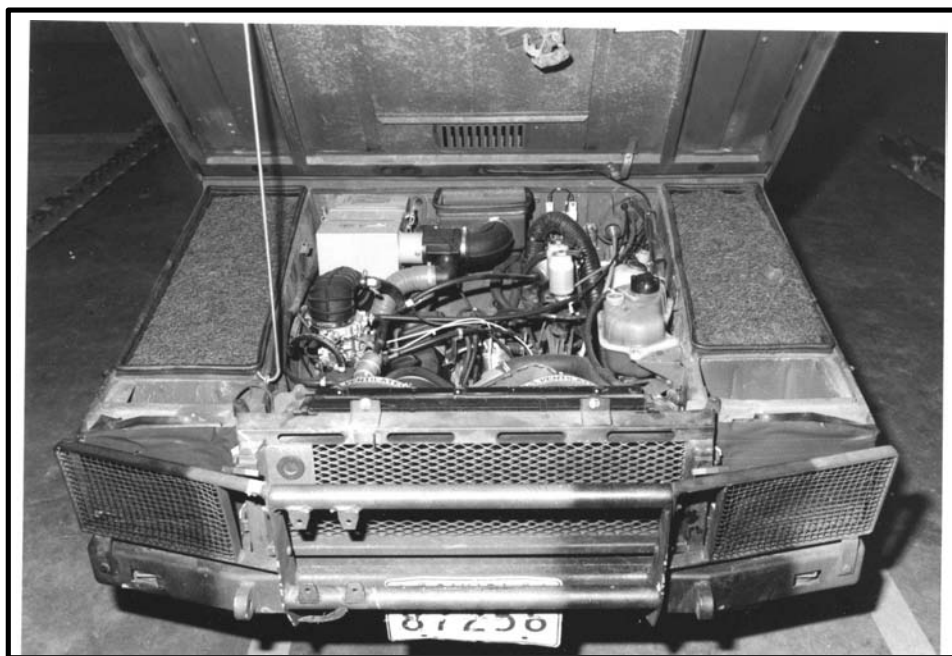
Figure 1-7 Tool Storage Wells – Excess Space Filled
