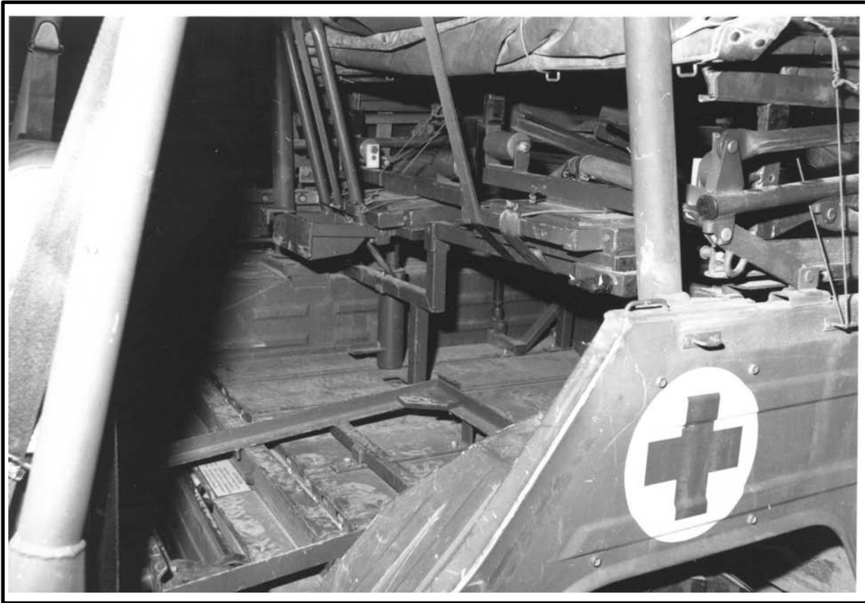
Figure 4-9 Stretcher Carrier Secured
