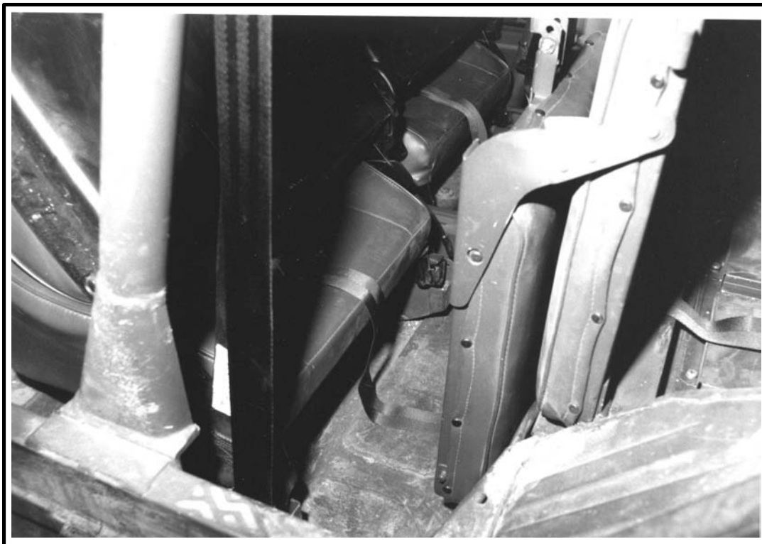
Figure 1-4 A7A Strap Routing Under Seats
