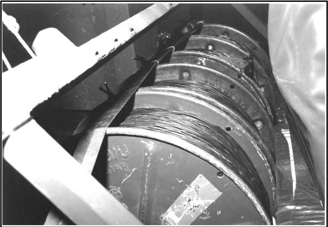
Figure 6-23 Honeycomb Between Reels and Door Bag
