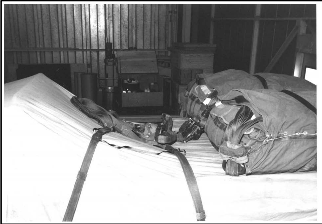
Figure 4-25 Suspension Slings Safe-tied
