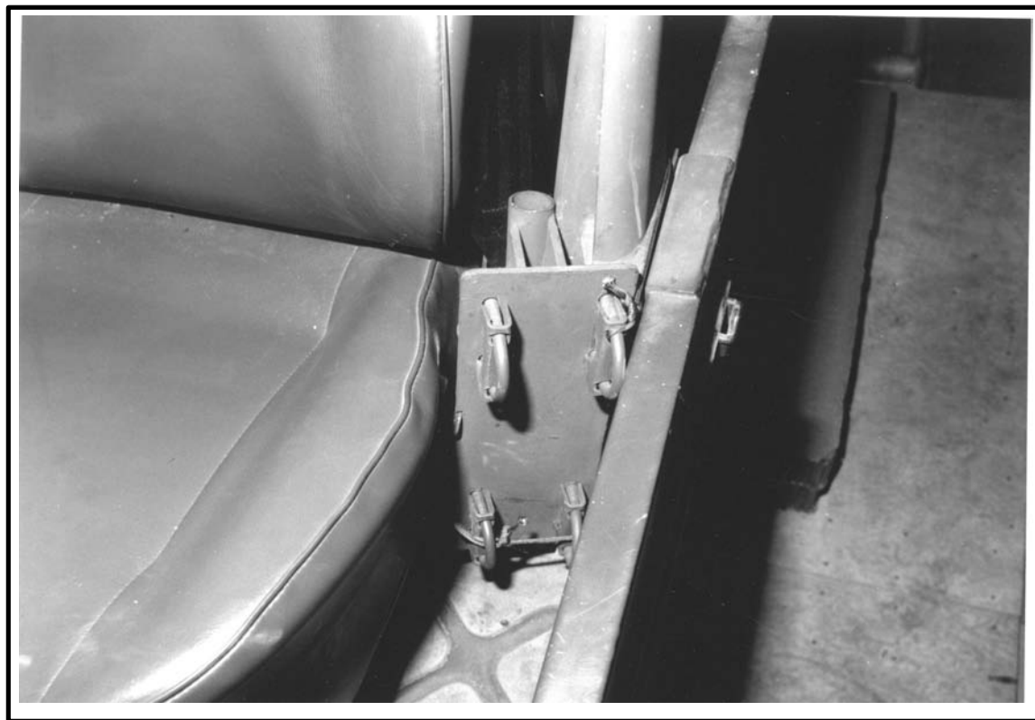
Figure 4-17 Wire Cutter Holder Secured
