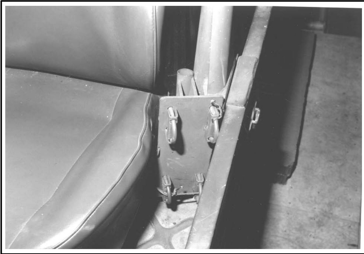
Figure 6-18 Wire Cutter Holder Secured
