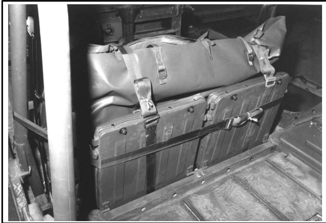
Figure 1-5 A7A Straps Installed (Rear View)
