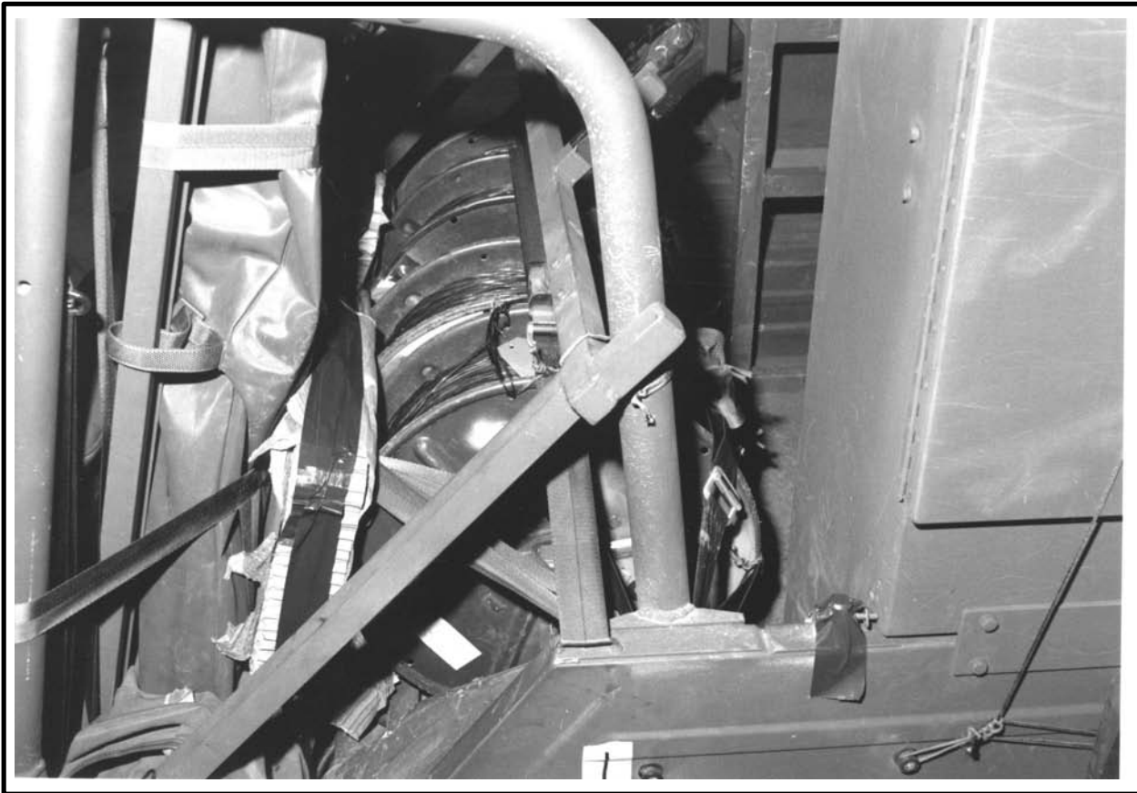
Figure 6-22 Reels Secured for Vertical Movement
