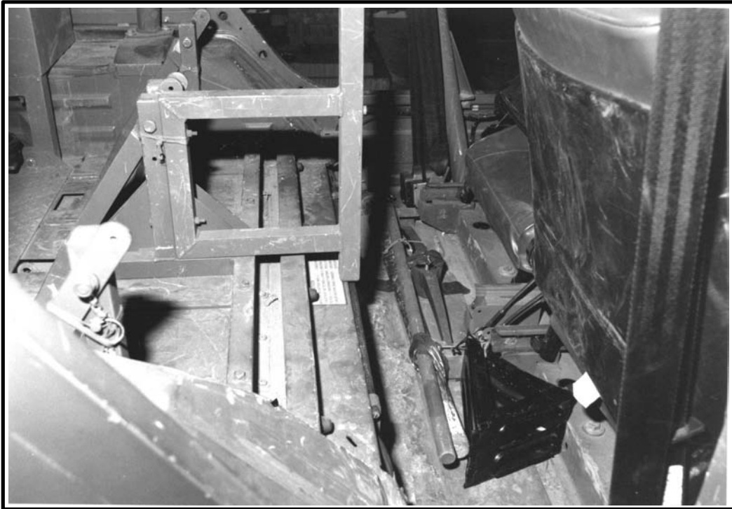
Figure 6-8 Pickhead, Pickhandle, Crookstick and Wheel Chock Secured
