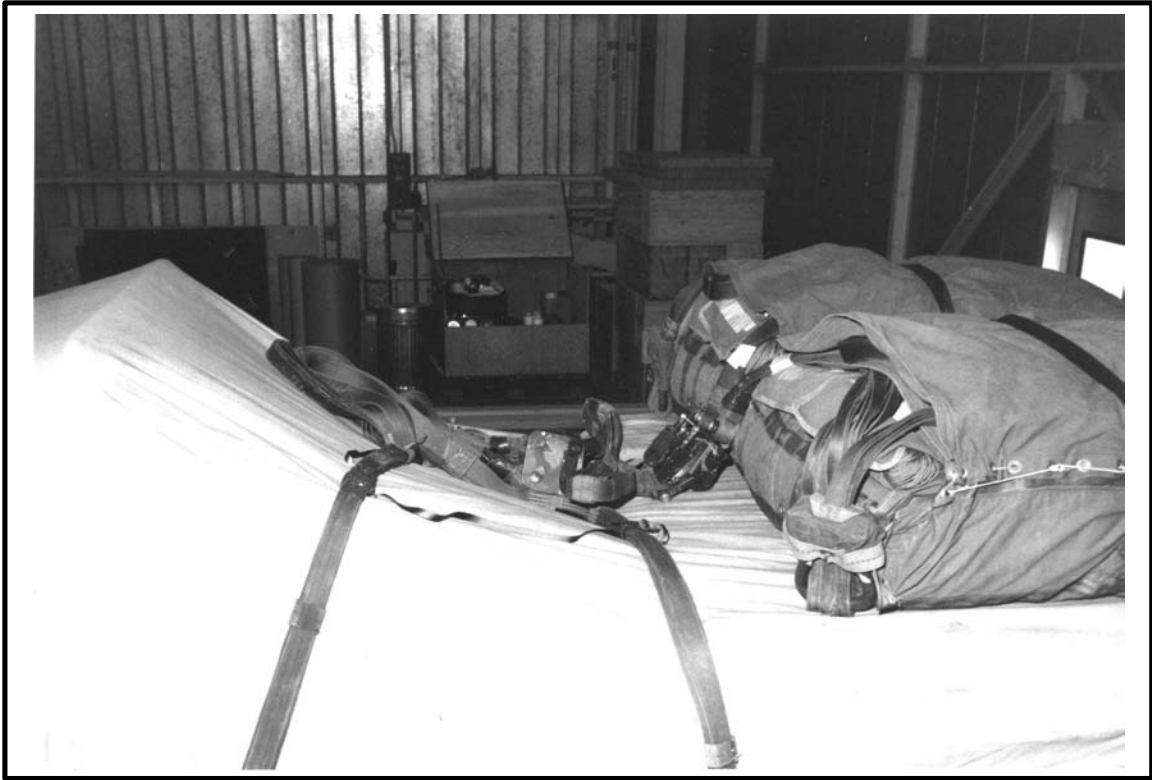
Figure 2-9 Suspension Slings Safe-tied
