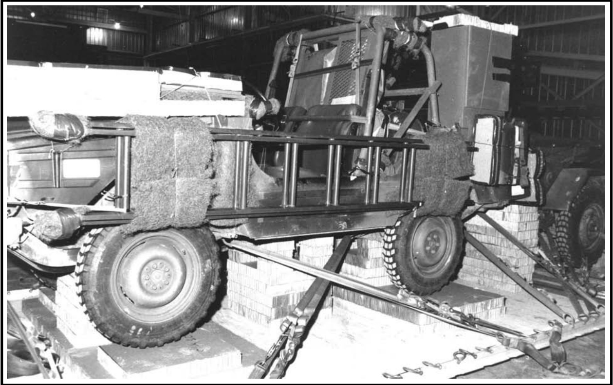
Figure 6-25 Ladder Secured in Position
