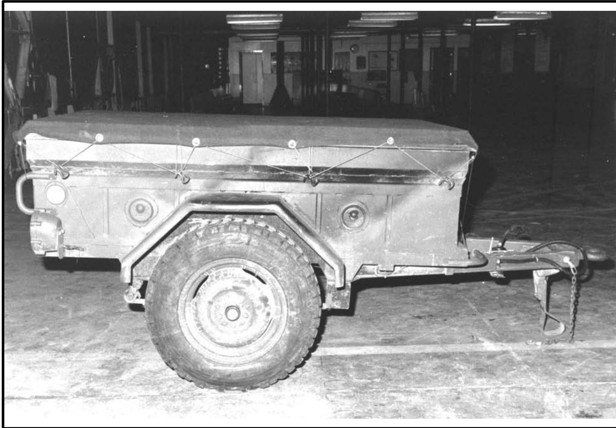
Figure 1-15 Canvas Cover Installed on Trailer
