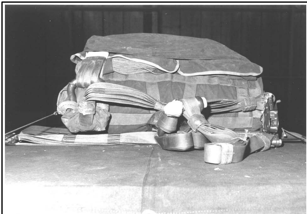
Figure 1-17 Parachute and Release Assembly Installed
